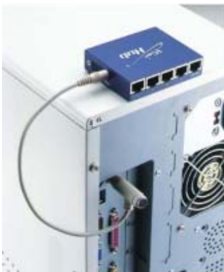
+5Vdc Power from Shared PS/2 Keyboard
