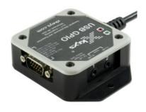
Trigger any action on a computer or tablet from a switch or 5 volt input, and/or send a 5 volt signal to any relay or circuit. The X-keys USB GPIO features ten configurable ports, two dedicated 5VDC outputs, and four dedicated short-to-ground inputs. The configurable ports can accept short-to-ground input, 5VDC input, or send 5VDC signal output.
