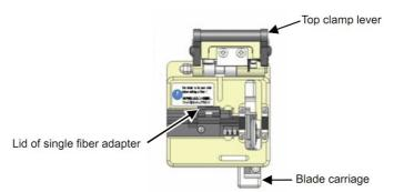
2. Lower the fiber straight into the correct V-groove with the end of the fiber coating (e.g. if the cleave length is 16mm) at the 16mm mark on the ruler.
