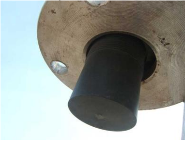
⑦ Screw the nut and fix the transducer
