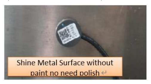
Step3: Test the installation point.
