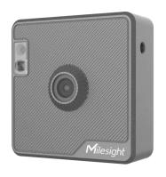
Milesight X1 Sensing Camera is a creative AloT product with applicable and intelligent applications. By capturing pictures, X1 Sensing camera can replace human inspection in multiple scenarios and economize on manpower. High-quality picture-capturing function and embedded supplement light make it more competitive and useful under different environmental conditions.
